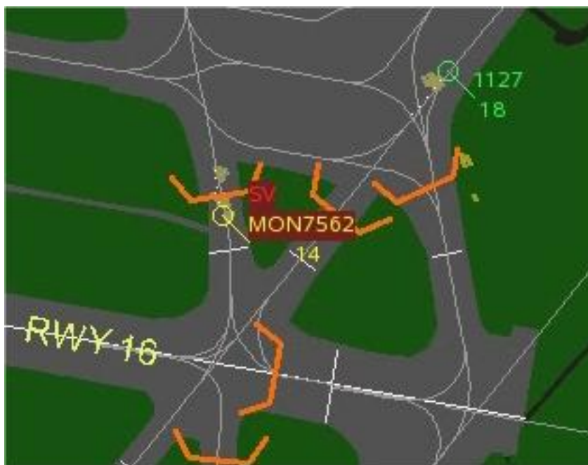
Figure No. 5: SVM Alert in Test Configuration
